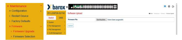
Following the upgrade the new firmware is immediately available. Any old firmware can very simply be re-activated in the menu "Firmware Selection" where the old firmware shall be applied again for some reason.
