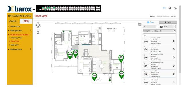
To position a camera or switch in a plan, all that needs to be done is to click on the respective device in the list to select it and then to position this device in the plan – done.
